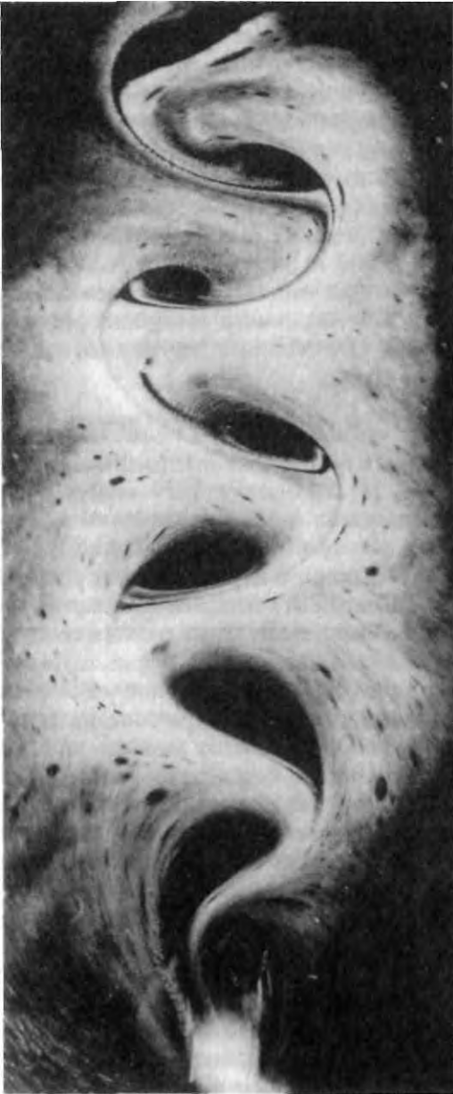
Water Disturbance Pattern. A thin brush has been drawn in a straight line through a shallow tray of glycerine treated water, whose surface has been dusted with powder. (Schwenk method, photo by A. J. Wilkes).
